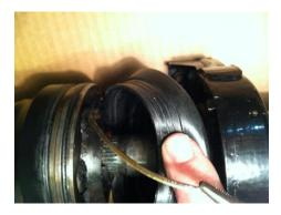
**Note:** Removal of this retaining key is the only way the splined sections of the shaft can be separated to allow servicing of the support bearing.
