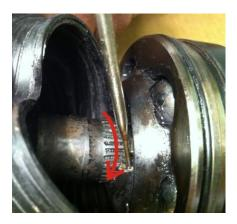
• Once a sufficient amount of the metal retainer key is exposed the remainder can be withdrawn with a pair of pliers.
