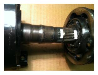
• Clean and lightly lubricate the splines and press together the shaft sections making sure to stop at the indexing paint mark.
