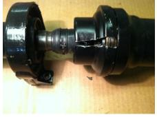
• A careful examination where the splined shaft enters the joint will reveal the retaining key way.
