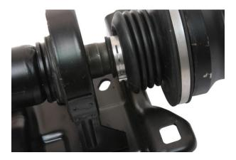
• The repaired shaft is now ready for reinstallation into the vehicle following the factory shop manual as a guide.
