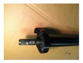
• Take short section of shaft containing the support bearing and press off the failed unit; then clean and press on the new support.
