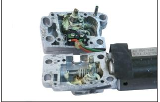
Reinstall the micro switch onto the cover. Move the lock lever from the fully open position to the fully closed position making sure the micro switch is activated at the very end of travel for each cycle. If necessary loosen the screw to move the activating cam to ensure this happens before fully tightening the set screw.
