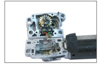
Install new drive gear / shaft assembly making sure it mates properly with motor pinion gear, taking care not to lose any of the distance shims under the old gear if present.
