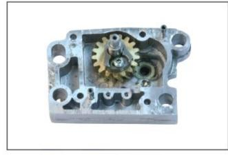
Ensure the locking lever is turned back to the open position and reinstall micro switch cam. Use the indexing marks made earlier to align the cam timing correctly,
