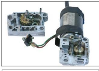
Carefully pry off upper cover exposing the gear set and miro-switch taking care not to change the lock arm position. <u>Note:</u> the locking arm will move freely once the gears disengage.
