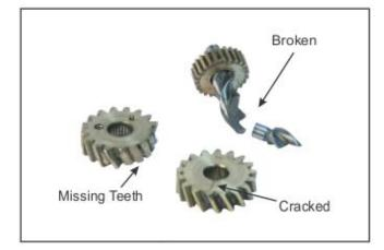
Both must be replaced and not only the damaged gear. The drive gear/shaft assembly and driven lever operating gear are subject to multiple types of failures.
