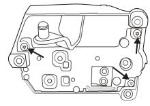
Step 3 – Remove upper shift cover (steel) attached by (2) T10 & T20 Torx screws.
