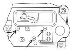
Step 2 – Remove outer aluminum cover attached by (3) T20 Torx screws.
