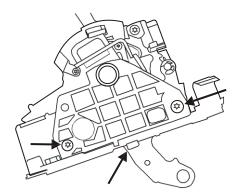
Step 5 – Remove park solenoid attached by (2) T25 Torx screws. Note: Two rivets may require drilling out in some instances; new ones are supplied in kit.
