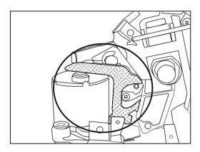
\*Note: there are 2 styles of shift park levers which are differentiated by the width of the hinge pivot base. Either a 5mm or an 11mm base may be fitted. This is a running change and not defined by a specific year or chassis. A quick inspection of the existing plastic lever in the shifter may be required before ordering the correct part.
