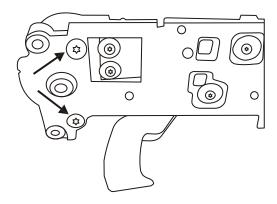
Step 6 – Using a suitable drift, remove fulcrum pin on remaining piece of broken plastic shift lever.
