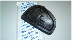
2. Reverse the wire harness boot. Push it entirely inside out with your finger making sure not to damage the rubber material.
