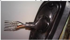
5. Reinstall wire pins in plug housing noting wire color order from earlier. Pull the wires back through in order to pull the plug housing back into position inside the slot in the gasket.
