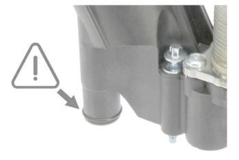
Warning: be careful inserting oil inlet pipe!
