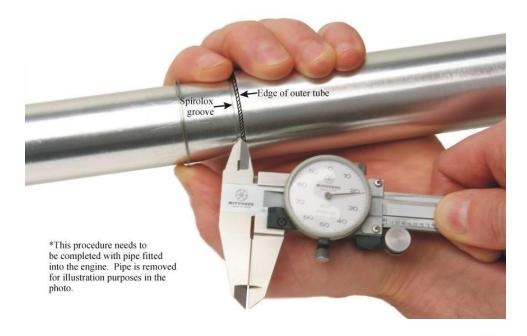
17. After re-seating the tube in the block and determining that the gap has been minimized, slide the pre-installed spiral lock ring into the groove.
