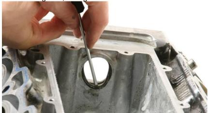
7. Carefully clean front seal galley. Lubricate all sides of new front seal with provided grease.
