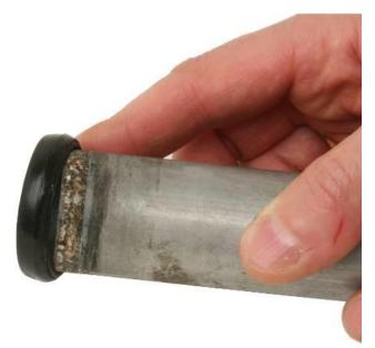
The original bonded seal fails primarily due to corrosion caused by an electro chemical reaction between the materials over time.
